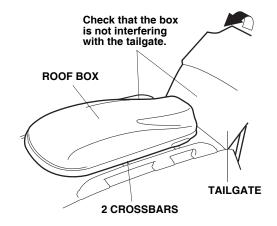
2. Open the roof box. Slide the plates forward or backward until the holes in the plates are over the front roof rack crossbar.
