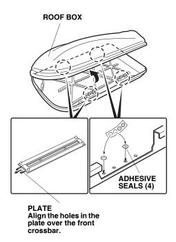
3. Attach adhesive seals over the unused rear mounting holes on the bottom of the roof box. The seals will help prevent water from entering the roof box. Remove the roof box from the vehicle.
