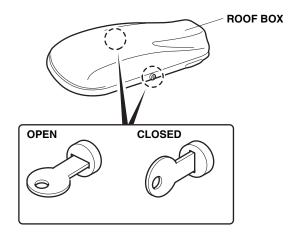
**Locking:** Press down on the lid. There should be an audible click. Be sure the lid is latched by attempting to lift the lid. Turn the key clockwise to lock the roof box. Remove the key while not in use. Make sure the straps do not dangle from the roof.
